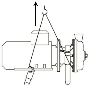
Remove the shroud before lifting!
